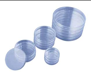
Stackable Thomas Petri Dishes are ideal for general laboratory use while Slippable Thomas Petri Dishes are designed for automated filling systems. Vented lids permit air circulation during incubation to reduce condensation build-up. Petri dishes are optically clear for easy viewing.
