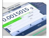
Intelligent functions, such as StatusLight, LevelControl and GWP Approved, help ensure right-first-time results by actively monitoring that all relevant conditions for correct weighing are met.
