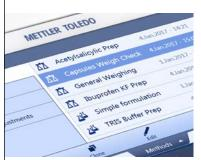
Process and balance settings for different weighing tasks can be saved on the balance as individual methods. Easily accessed, users have a quick and convenient way to start tasks and every user follows the same procedure.
