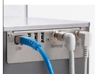
Multiple interfaces (4 USB, 1 LAN) provide error-free data transfer and many connection possibilities. XPR balances automatically recognize and configure a connected device in seconds, enabling you to get started right away.
