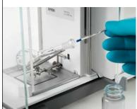
By dosing directly into your tare container, you avoid the tedious back-weighing and recalculation processes associated with sample transfer via e.g. weighing paper—and you don't lose any of your precious samples.
