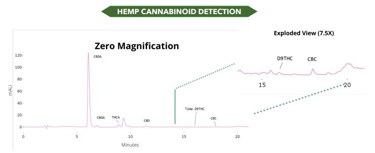
UV detection of 5 cannabinoids in a hemp-variant of cannabis at 235 nm using the Axcend Focus LC. Elution Order – 6.5 min: CBDA; 7 min: CBGA; 8.5 min: THCA; 11 min: CBD; and 18 min: CBC. Flow rate: 0.97 μL/min; Gradient %B: 0 min–3%, 1 min–25%, 10 min–25%, 17 min–60%, 18 min–95%, 20 min–95%; Equilibration Time: 4 min; Mobile Phase A (50% H<sub>2</sub>O 50% ACN 0.3 M NH4Ac buffer pH 4.6); Mobile Phase B (50% MeOH 50% ACN); Column: 10 cm x 150 μm i.d.; Phenomenex Kinetex 1.7 μm C8.
