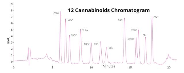
UV detection of 12 cannabinoids in a Restek standard at 235 nm using the portable Axcend Focus LC. Elution Order shown above and below. Flow rate: 0.97  $\mu$ L/min; Gradient %B: 0 min–3%, 1 min–25%, 10 min–25%, 17 min–60%, 18 min–95%, 20 min–95%; Equilibration Time: 4 min; Mobile Phase A (50% H<sub>2</sub>O 50% ACN 0.3 M NH4Ac buffer pH 4.6); Mobile Phase B (50% MeOH 50% ACN); Column: 10 cm x 150  $\mu$ m i.d.; Phenomenex Kinetex 1.7  $\mu$ m C8. (See table below for more details.)
