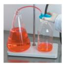
While holding the VacuCap device securely on the filtrate container, start the vacuum.
