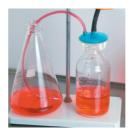
4. When filtration is complete, switch off the vacuum pump allowing the vacuum inside the receiving container to dissipate. Refer to the product insert for complete instructions.
