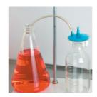
Connect the feed tubing to the port marked "INLET" on the VacuCap device. Place the opposite end of the tubing in the unfiltered fluid to be drawn.
