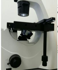
3.5 watt LED with dimmer control lasts 10,000 hours Clean look leads to smooth operation, focus/light control
